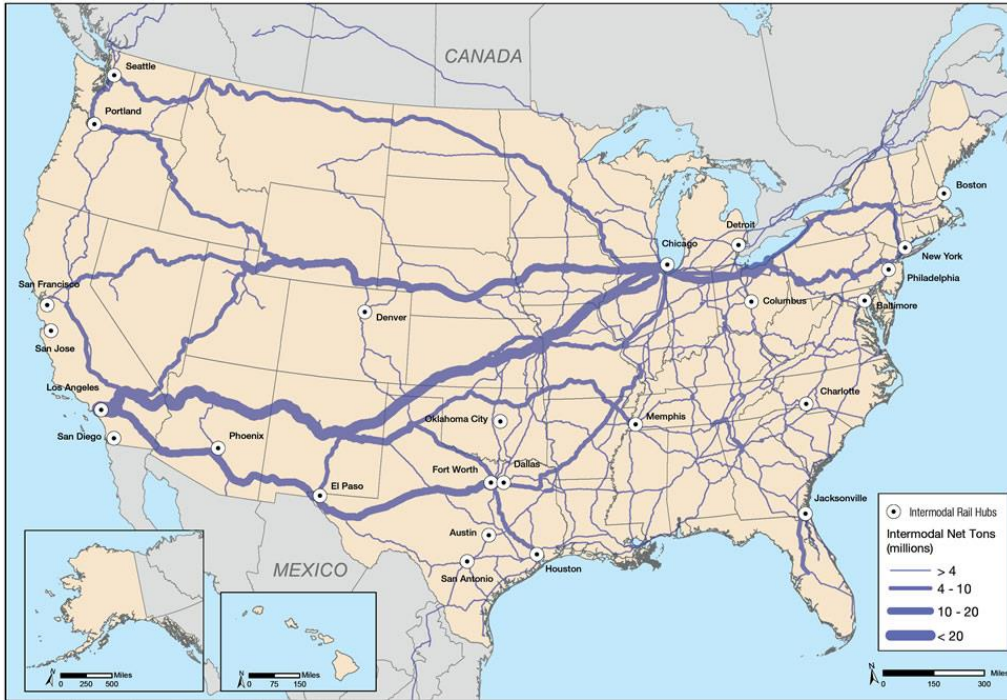
Figure 12 2011 U.S. Intermodal Freight Rail Network and Volume for TOFC and COFC (USDOT/FHWA, 2013)
